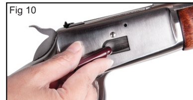
Fig 10 Gun being loaded through the loading port
