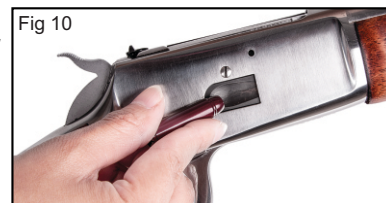
Fig 10 Gun being loaded through the loading port
